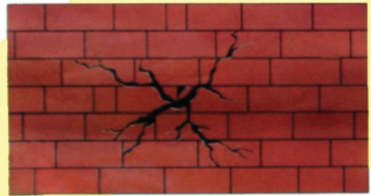
CRACK THROUGH ONE BRICK, THE WALL IS DAMAGED
